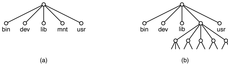
Figure 1-22. (a) File system before the mount. (b) File system after the mount.
